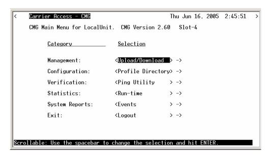
**WARNING!** THE CMG ROUTER WILL RETURN TO DEFAULT VALUES IF THE CODE IS DOWNGRADED TO A RELEASE PREVIOUS TO 2.10.
